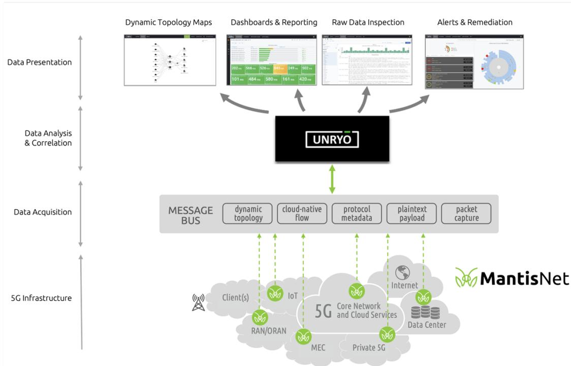
Figure 1: The Mantisnet/Unryo Platform
